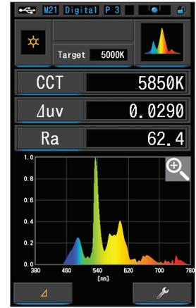
The Spectrum screen displays the spectral energy distribution of a source in real time. It can be displayed as a graph and data or full screen.
