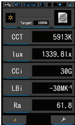
The TEXT screen displays user selected measurement values. Real time measurements appear and are updated after every reading, next to their light measurement values.
