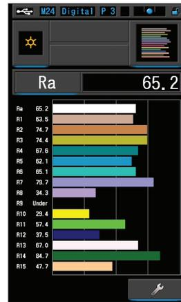
The CRI screen displays the standard color reference values (including R1 thru 15) as a percentage of the light sources ability to reproduce a color accurately, as compared to the Ra standard.
